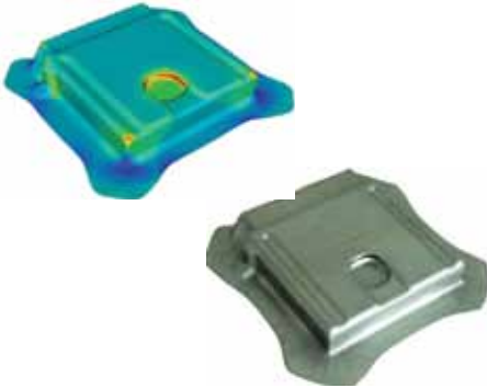
Simulation Results Accurately Predict Part Failure
